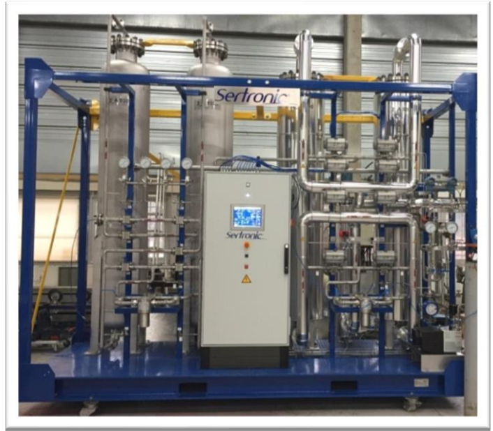
Helium dryer 600 Nm 3 /h - 30 Barg
