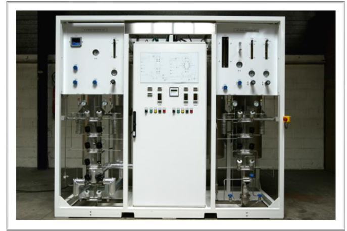
Nitrogen dryer 20 Nm 3 /h -230 Barg & Argon purifier 15 Nm 3 /h – 15 Barg
