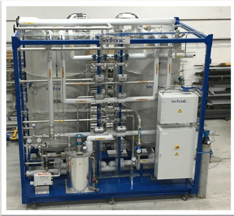
Helium cryogenic purifier 500 Nm 3 /h - 380 Barg
