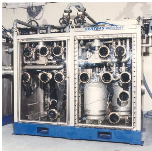
Tritium removal unit 250 Nm 3 /h – AP
