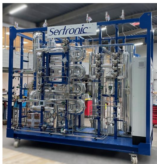
Hydrogen purification unit DS 2000-85
