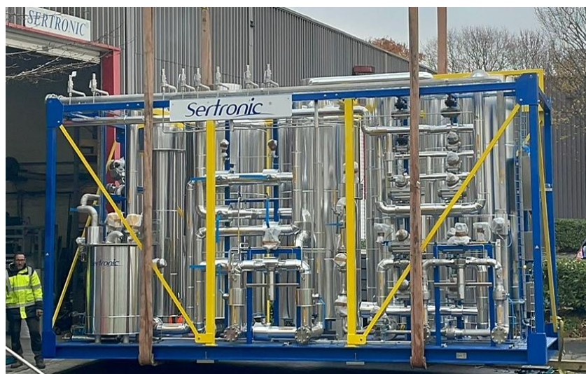
Hydrogen purification unit DS 4000-45
