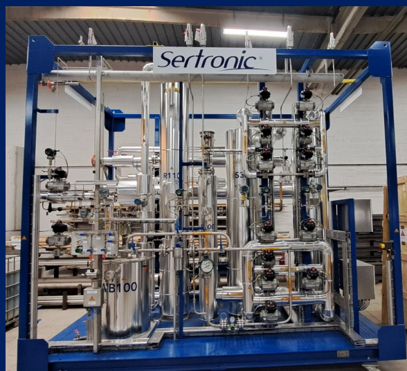
Hydrogen purification unit DS 2000-90
