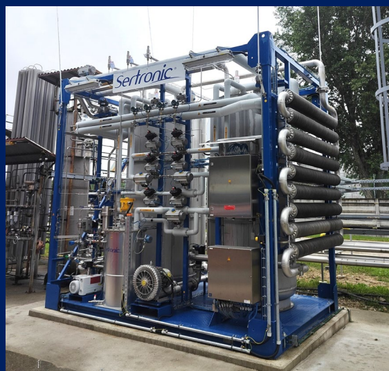
Hydrogen cryogenic purifier EF 1500-250
