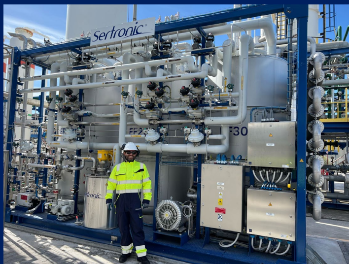
Hydrogen cryogenic purifier (3 columns) EF 1000-15
