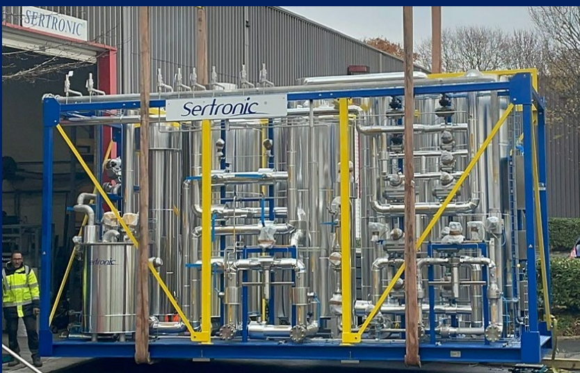
Hydrogen purification unit DS 4000-45
